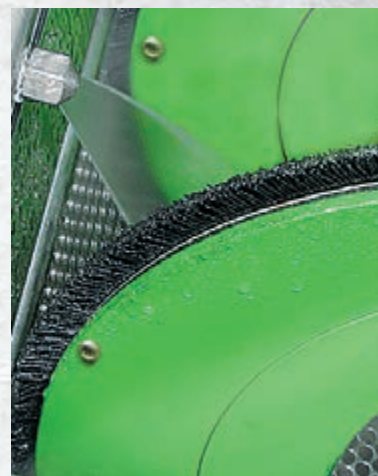
Replaceable auger brush keeps perforated screen clean and helps transport solids
