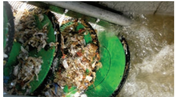
Solids captured and removed by auger
