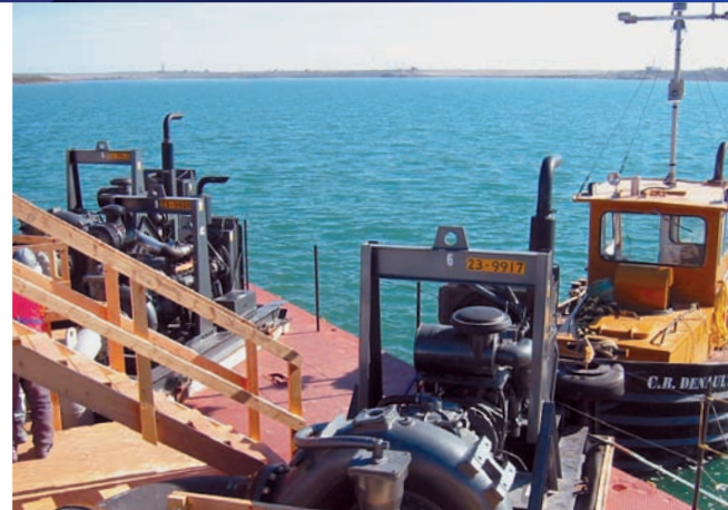
THE 16NHG22's EMPLOYED ON TWO BARGES.
