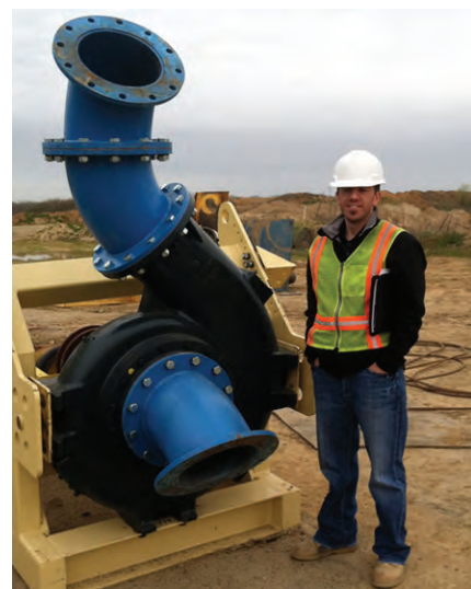
THE CORNELL 12NHTB RESTING NEAR THE AGGREGATE PIT, WAITING TO BE INSTALLED ON THE BARGE
